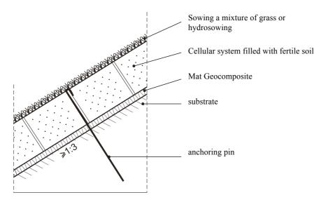
Grass seeds are introduced on slope surfaced covered with humus with use of traditional sowing or hydrosowing. On reinforcements where it is required to obtain turf cover very soon, grass in rolls may be installed.
