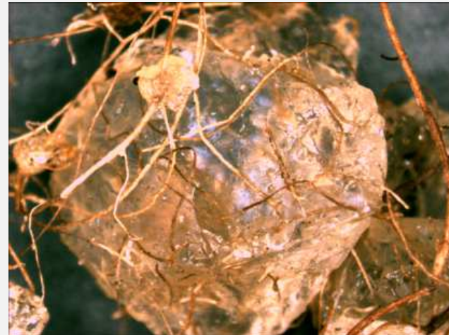
SAP overgrown by roots
